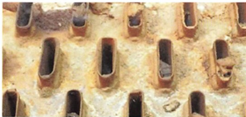
Fig. 5. My radiator that was tanked only. Radiator was still about 1/3 restricted.
