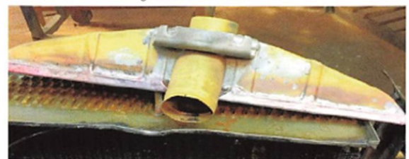
Fig. 8. Top ready to be soldered
